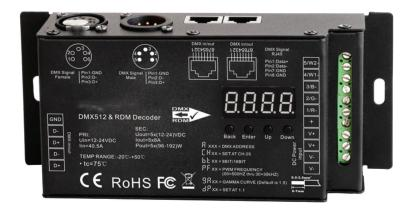
The DR-DMX-5CH-DEC is a 5 channel digital decoder that allows a DMX controller to tell your color changing LED load what to do. You can either hard wire your DMX connections or choose from XLR DMX or RJ45 cables to communicate from your DMX controller to the decoder. Each decoder will require a 12VDC or 24VDC driver to power the load it handles.
