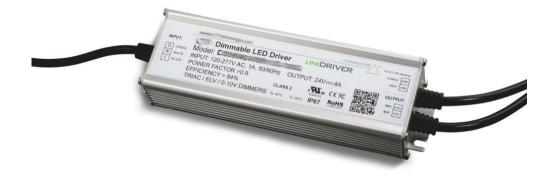
The universal series driver is aone size fits all solution for indoor and outdoor lighting applications. Universal input of 120-277V, universal phase dimming (forward and reverse) to 1%, as well as 0.1% dimming in 0-10V. This driver truly is universal.
