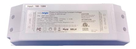
These drivers are rated for dry and damp locations. Universal phase dimming capability allows for the use of both forward and reverse phase dimmers. TRIAC, MLV, and ELV dimmers will all work. Rated for 100-130V input and outputs of 24W, 48W, and 60W, these drivers are great for low wattage applications in dry and damp locations. The DIMA series drivers come with a 3 year warranty.
